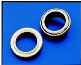
Mechanical seal: Tungsten carbide rotating and stationary seal faces with Viton elastomers with 304 stainless steel sleeves; grease or oil lubricated which allow the pump to run dry & operate on high vacuum even while pumping abrasive liquids.
