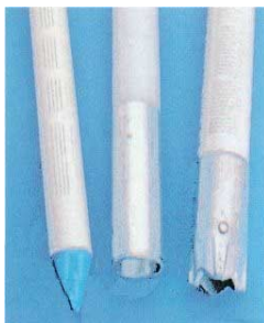
Wellpoint Used to draw air and water from under ground to temporarily lower the water table in a limited area and allow for construction. Self jetting, stainless steel with PVC screens, or all PVC Wellpoints are available.
