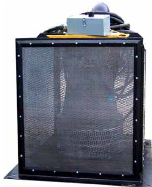
The Thompson 6-inch Compressor-Assisted Dry-Prime pump recirculated the acidic water and lime mixture to maintain pH levels.
