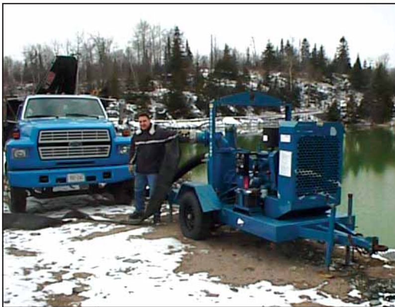
Fig. 2: Sam Scola, INCO Limited, Sudbury Operations stands by his Thompson 6-inch Compressor-Assisted Dry-Prime Pump.
