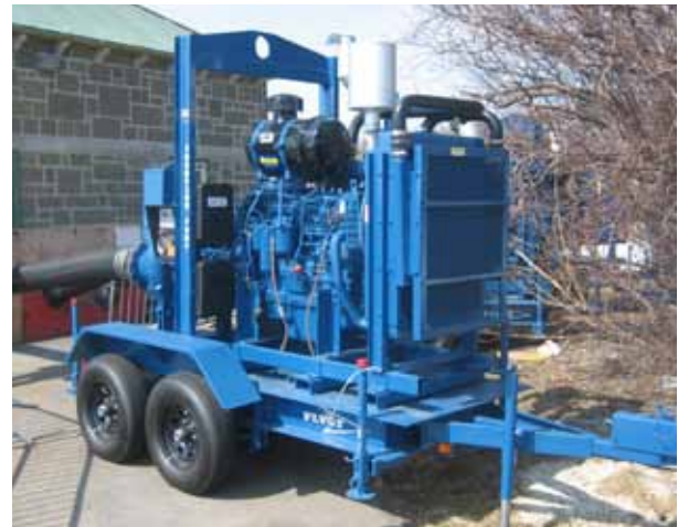
Trailer-mounted, self-priming Thompson model 12JSCG-DJDST-81H-M pump.
