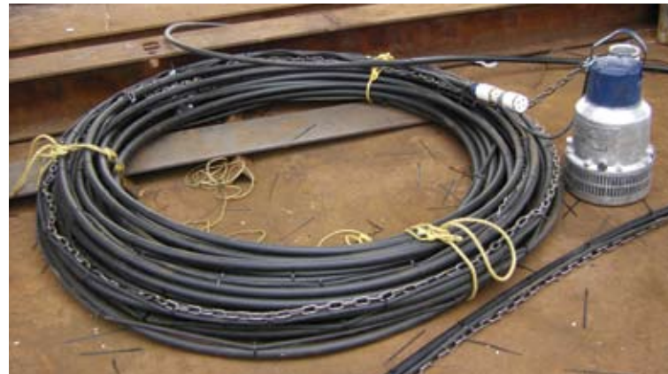
A BS 2125 pump with the specially ordered 400-foot long cable.
