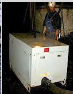
SV300 pump with one man transfers 30 m 3 /h of muck and 3" rock with a 4" hose at underground mine. Supavac systems to >60 m 3 /h.
