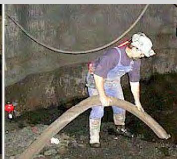
SV300 pump with one man transfers 30 m 3 /h of muck and 3" rock with a 4" hose at underground mine. Supavac systems to >60 m 3 /h.
