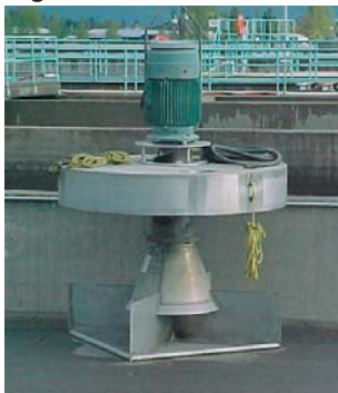
One of the surface aerators removed from Digester No. 1
